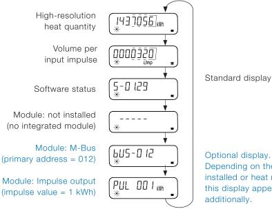
Optional display. Depending on the module installed or heat meter type, this display appears
