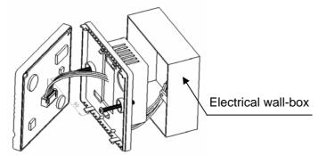
Screw terminals for 2 x 1.5 mm<sup>2</sup> or 1 x 2.5 mm<sup>2</sup>, min. ( 0.5 mm<sup>2</sup> )
